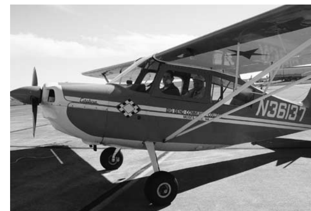
Students gain tail wheel experience with the college's Citabria. This plane is also used for spin training for flight instructors.
